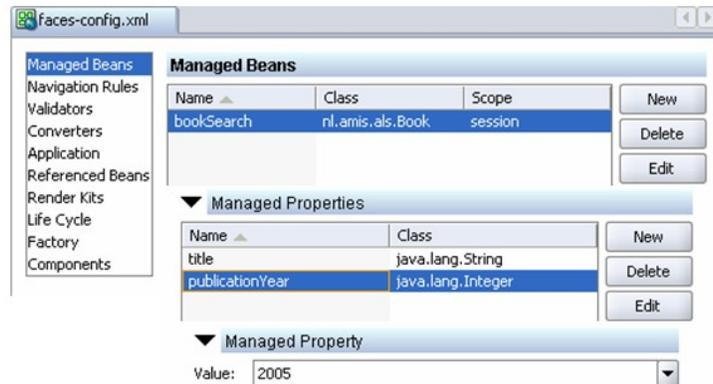
Figure 2 – Managed Beans and the JSF faces-config Console
