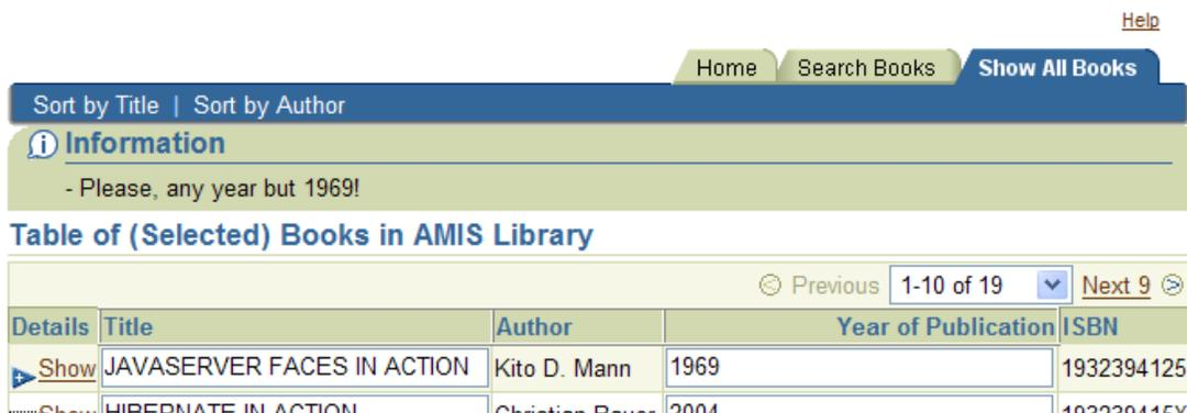
**Figure 7 – AJAX style immediate server side validation when Year field is changed**
